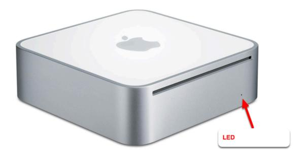
The early-2009 model Mac Mini is silver with a white top and includes a built-in DVD drive (see above). There are no other physical buttons or ports on the front other than a white LED in the bottom that indicates that the computer is turned on (glows white when on), or asleep (flashes slowly when asleep).
