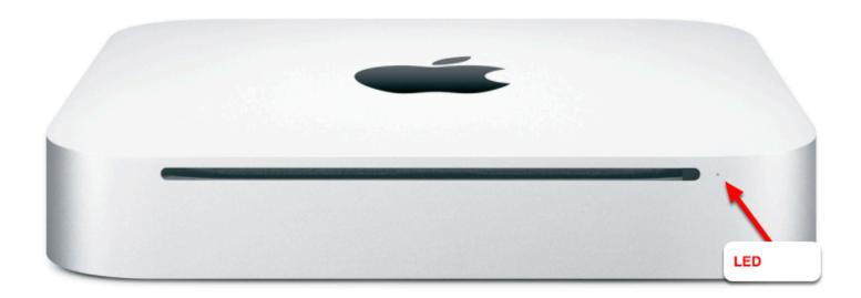
The Mid-2010 model Mac Mini is all silver with a black back panel and includes a built-in DVD drive (see above). There are no other physical buttons or ports on the front other than a white LED in the bottom that indicates that the computer is turned on (glows white when on), or asleep (flashes slowly when asleep).
