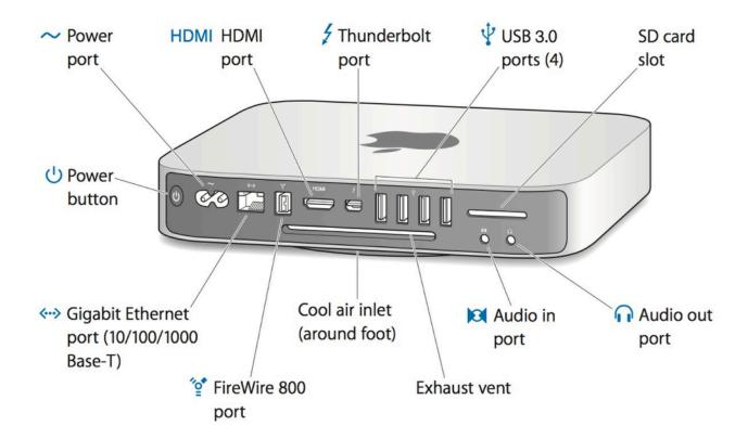
The rear of the Mac Mini houses all of the ports, the power switch, and power connector. Ports available on the 2012 Mac Mini including:
