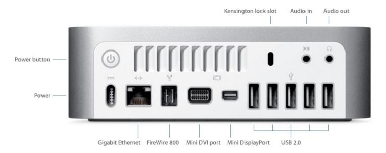
The rear of the Mac Mini houses all of the ports, the power switch, and power connector. Ports available on the 2009 Mac Mini including:
