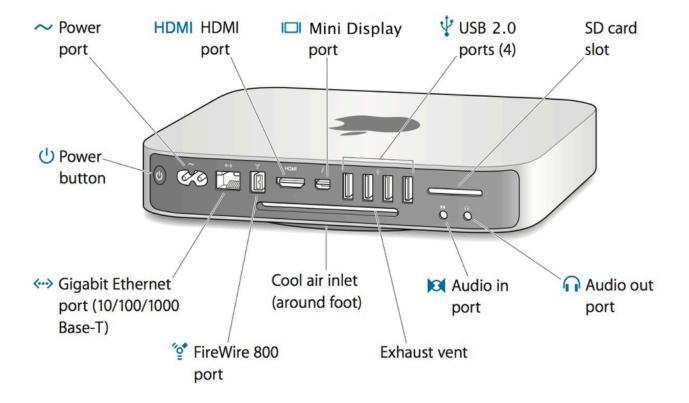
The rear of the Mac Mini houses all of the ports, the power switch, and power connector. Ports available on the 2010 Mac Mini including:
